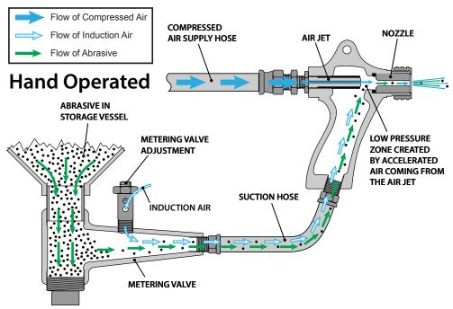
**Automated** COMPRESSED NOZZLE AIR JET **AIR SUPPLY HOSE Machines** METERING VALVE ADJUSTMENT ABRASIVE IN STORAGE VESSEL **SUCTION HOSE** LOW PRESSURE INDUCTION AIR ZONE CREATED BY ACCELERATED AIR COMING FROM THE AIR JET
